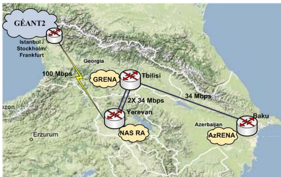
Figure. 2 Centralized BSI Network Topology with Armenia being the center
